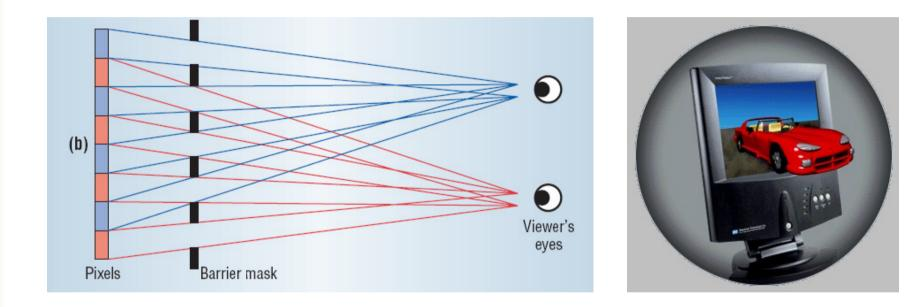
A barrier mask is placed in front of the pixel raster so that each eye sees light from only every second pixel column (left); 2D/3D switchable autostereoscopic display from DTI
