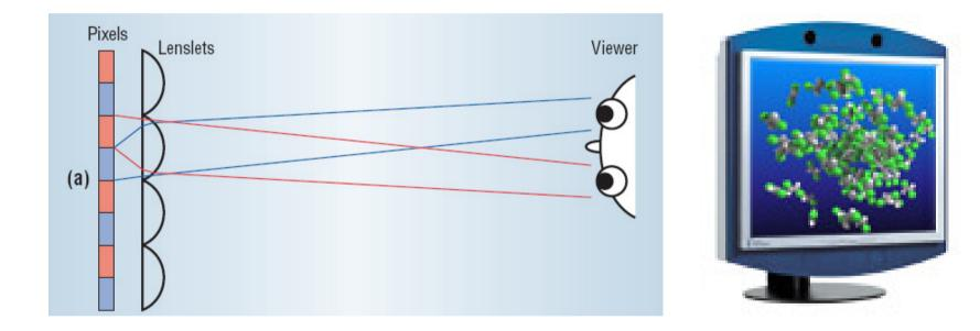
An array of cylindrical lenslets is placed in front of the pixel raster, directing the light adjacent pixel columns to different viewing slots so that each of the viewer's eye sees light from only every second pixel column
