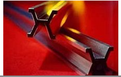
Historical International Prototype Meter bar, made of an alloy of platinum and iridium, that was the standard from 1889 to 1960.
