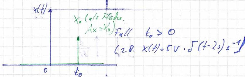
$$A_x = \int_{-\infty}^{+\infty} x_0 \cdot \delta(t-t_0) dt = x_0 \int_{-\infty}^{+\infty} \underbrace{\delta(t-t_0)}_{1} dt = x_0$$
