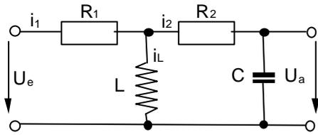
$$T_0^2 \cdot \ddot{u}_a(t) + 2dT_0 \cdot \dot{u}_a(t) + u_a(t) = T_D \cdot \dot{u}_e(t)$$
