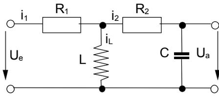
$$T_0^2 \cdot \ddot{u}_a(t) + 2dT_0 \cdot \dot{u}_a(t) + u_a(t) = T_D \cdot \dot{u}_e(t)$$
