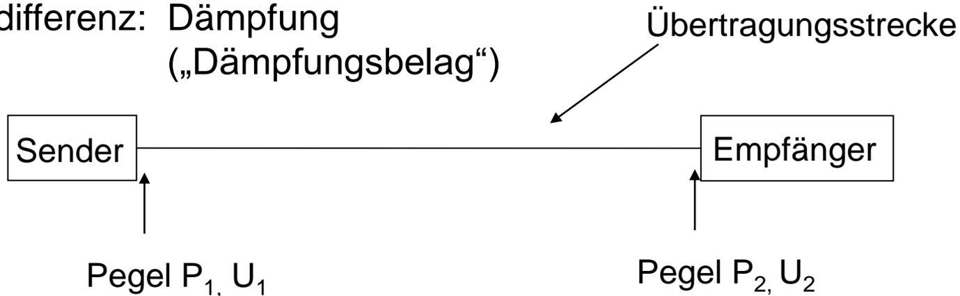
$$\Delta P_{\text{dB}} = 10 \log \left( \frac{P_{1[\text{lin}]}}{P_{2[\text{lin}]}} \right) \text{dB} = P_{1[\text{dBm}]} - P_{2[\text{dBm}]}$$
