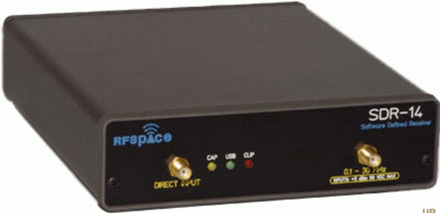
The image shows the RFspace SDR-14 Software Defined Receiver, a black rectangular device. The front panel features the RFspace logo on the left, a 'DIRECT INPUT' jack, three indicator lights labeled 'CAP', 'USB', and 'CLIP', and a '0.1 - 30 MHz' jack on the right. The text 'SDR-14 Software Defined Receiver' is printed on the top right of the front panel. Below the device, the letters 'UR' are visible.
