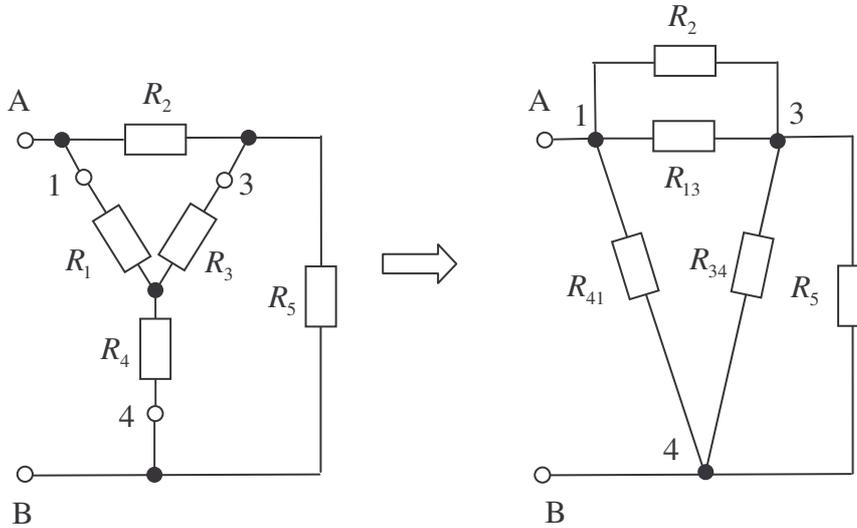
$$\underline{R_{13}} = \frac{280}{3} \Omega \approx 93,3\Omega \quad \underline{R_{34}} = 28\Omega \quad \underline{R_{41}} = 140\Omega$$
