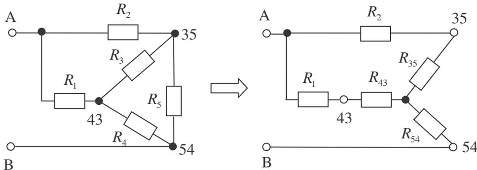
$$\underline{R_{35} = \frac{160}{41}\Omega \approx 3,9\Omega} \quad \underline{R_{54} = \frac{240}{41}\Omega \approx 5,85\Omega} \quad \underline{R_{43} = \frac{150}{41}\Omega \approx 3,66\Omega}$$
