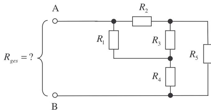
Werte:  $R_1 = 50 \Omega$     $R_2 = 40 \Omega$     $R_3 = 10 \Omega$
