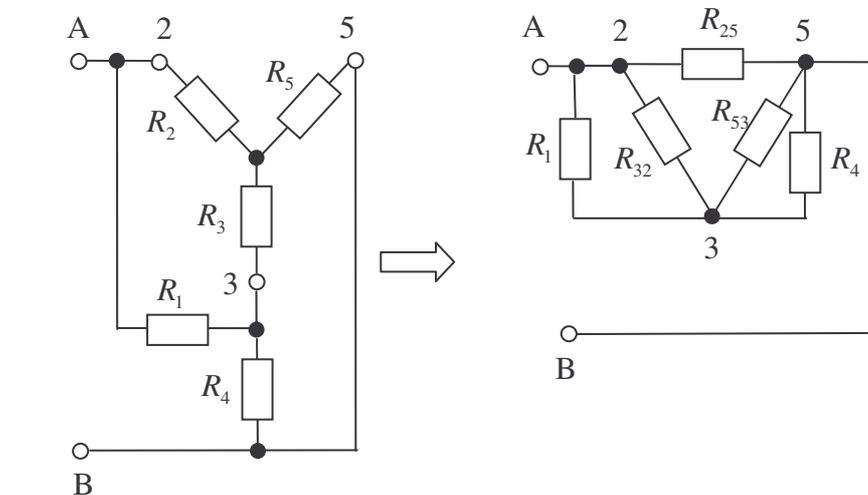
$$\underline{R_{32} = 75\Omega} \quad \underline{R_{25} = 120\Omega} \quad \underline{R_{53} = 30\Omega}$$
