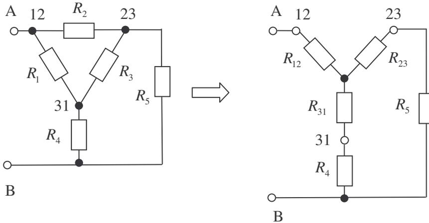
$$\underline{R_{12} = 20\Omega} \quad \underline{R_{23} = 4\Omega} \quad \underline{R_{31} = 5\Omega}$$
