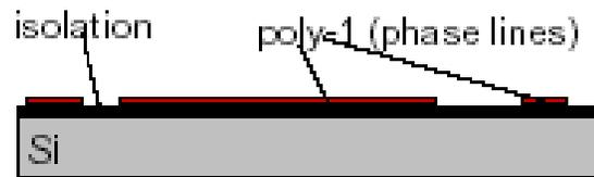
**step 1:** definition of phase lines by LPCVD-deposition and patterning of polysilicon on an isolating  $\text{Si}_3\text{N}_4$  layer.
