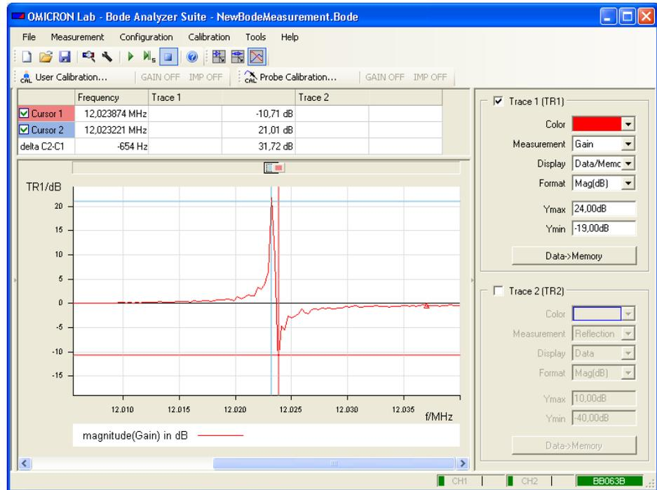
If the curve is above the 0 dB line the current measured data is higher than the stored measurement data. If the curve is below the 0 dB line the currently measured data is below the stored measurement data
