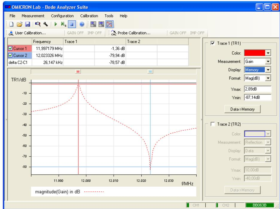
5. In the **Display** list, select **Data & Memory**, and then touch the housing of the quartz filter with your finger.
