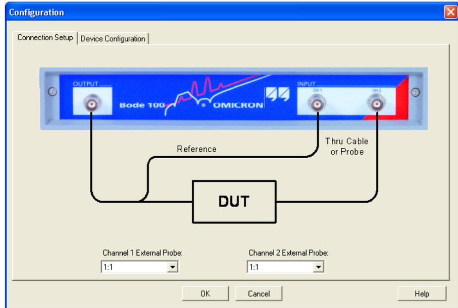
This picture shows how to connect the DUT.
