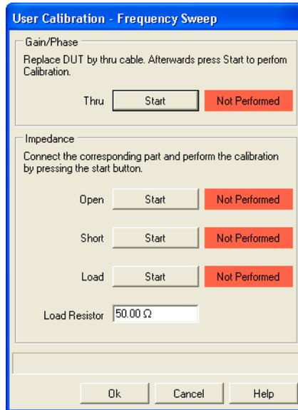
6. Connect the cable you want to use for the measurement to the OUTPUT connector of the *Bode 100*. Plug the BNC straight adapter on the other end of the cable to have the same reference plane.
