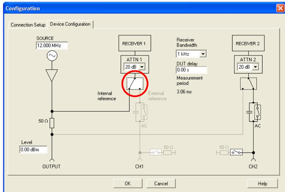
**Note:** The source signal is internally connected to the channel 1 input in front of the 50  $\Omega$  source resistor (channel 1 voltage  $V_0$  as defined in 3.1 "Basics" on page 20).
