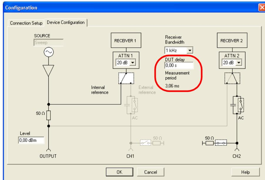
The measurement period indicates the time the *Bode 100* requires to perform measurement at one frequency point. By multiplying this value with the selected number of measurement points you can get an estimate of the expected sweep time.
