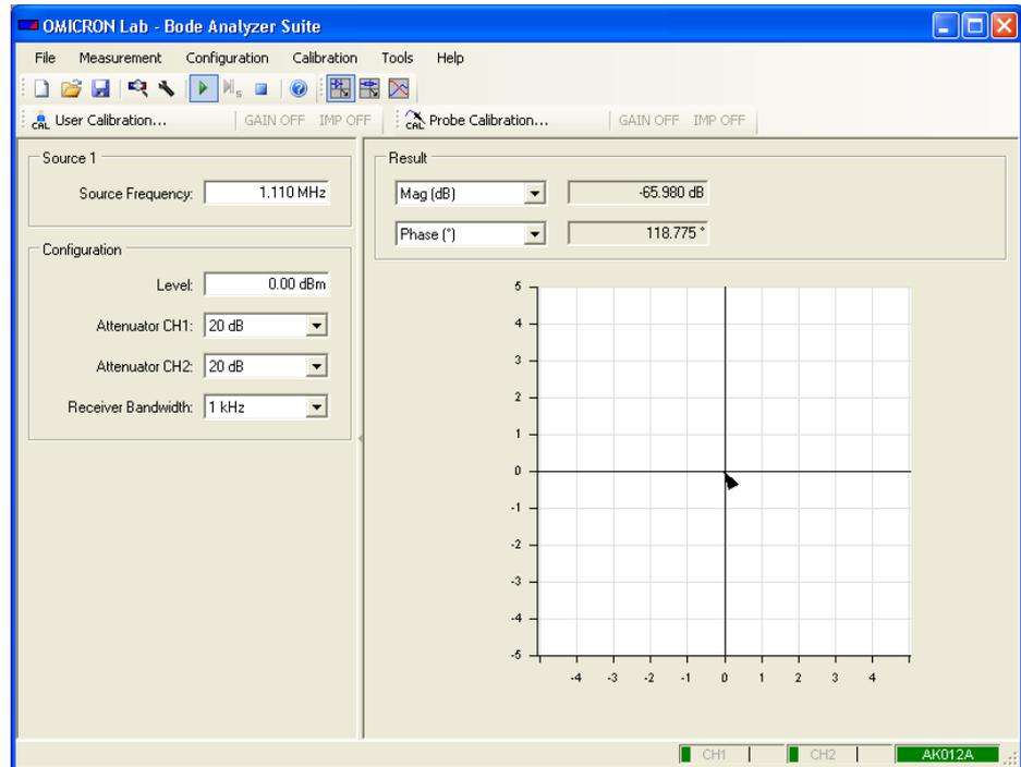
**Hint:** If you see a serial number e.g. AK001E in the status bar on the lower right side of the window then the *Bode Analyzer Suite* communicates with the *Bode 100*. If you cannot see the serial number check whether your *Bode 100* is connected and powered properly, and then click the
