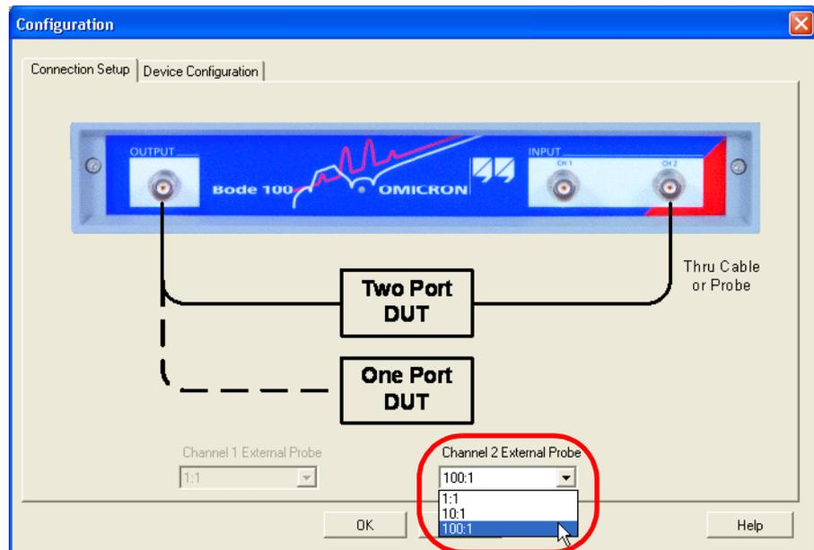
2. Ensure that your DUT is terminated correctly.
