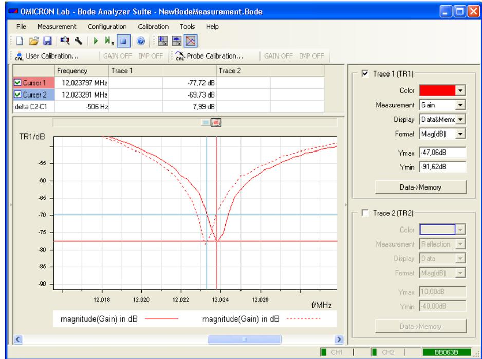
**Result:** Touching the quartz housing shifts the parallel resonance frequency by 506 Hz. You might measure different values with your quartz filter.
