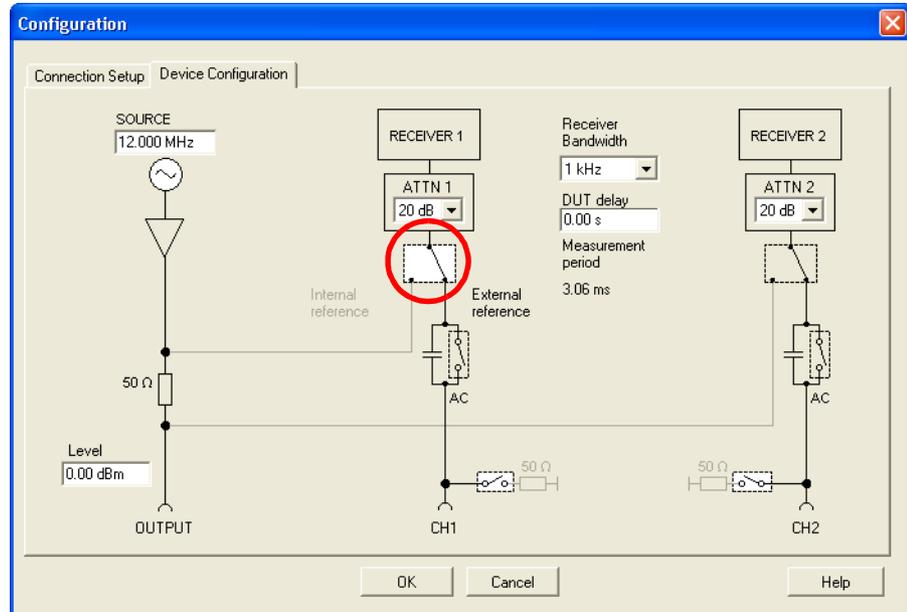
**Note:** The source signal is externally connected to the channel 1 input behind the 50 Ω source resistor (channel 1 voltage  $V_{IN}$  as defined in 3.1 "Basics" on page 20).
