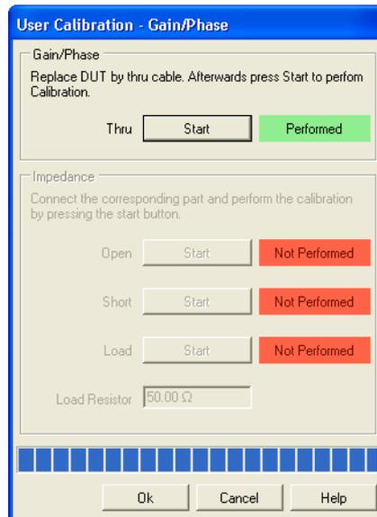
The calibration takes only a few seconds. The **Gain/Phase** mode is now calibrated for the current specific measurement setup.
