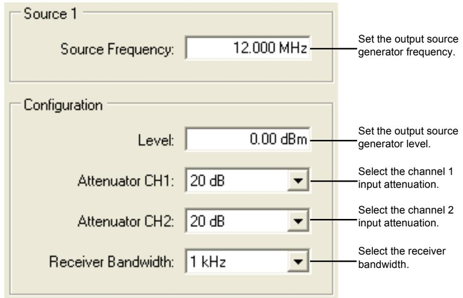
**Hint:** A higher receiver bandwidth allows faster measurements, a lower receiver bandwidth increases the measurement accuracy.
