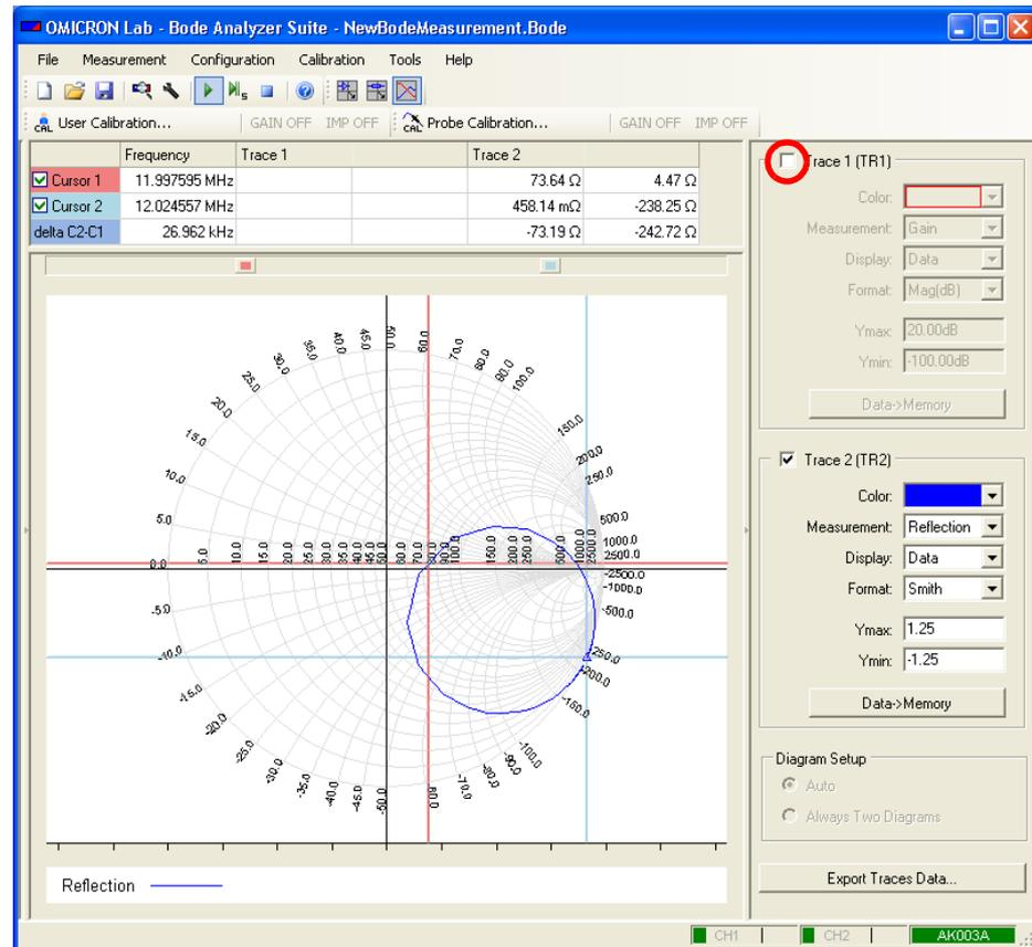
Since the output of the DUT (quartz filter) is connected to the channel 2 input, the measured impedance is the quartz impedance plus the  $50\ \Omega$  input impedance of the *Bode 100*.
