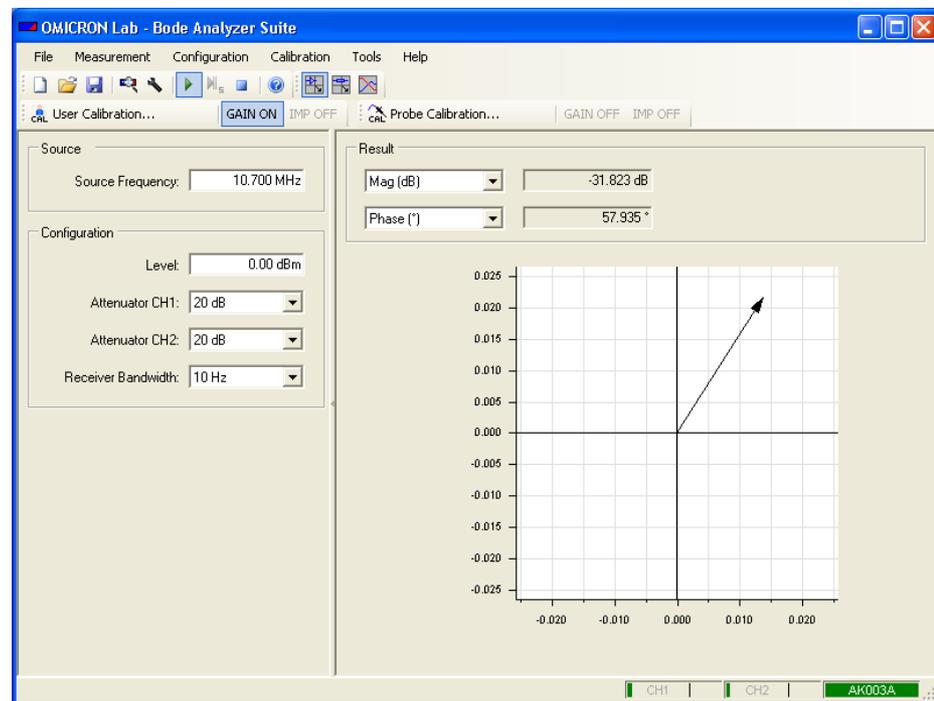
**Result:** The transfer function of the IF filter has a magnitude of  $-31.82$  dB and a phase shift of  $57.9^\circ$  at 10.7 MHz.
