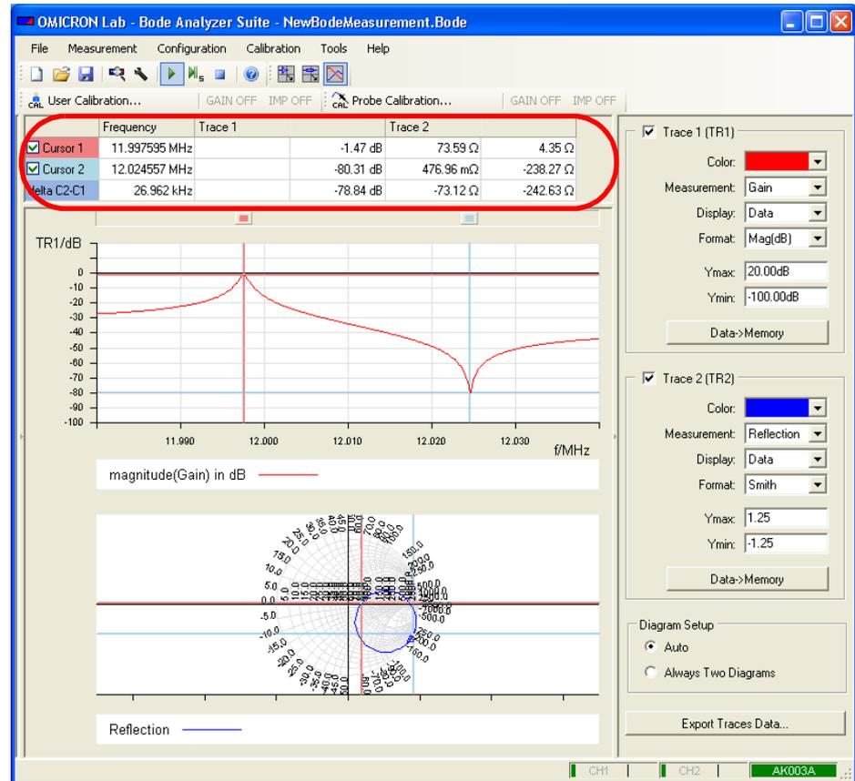
**Results:** Cursor 1 marks the series resonance frequency of 11.998 MHz and an attenuation at the series resonance frequency of 1.47 dB. Cursor 2 marks the parallel resonance frequency of 12.025 MHz and an attenuation at the parallel resonance frequency of 80.31 dB.
