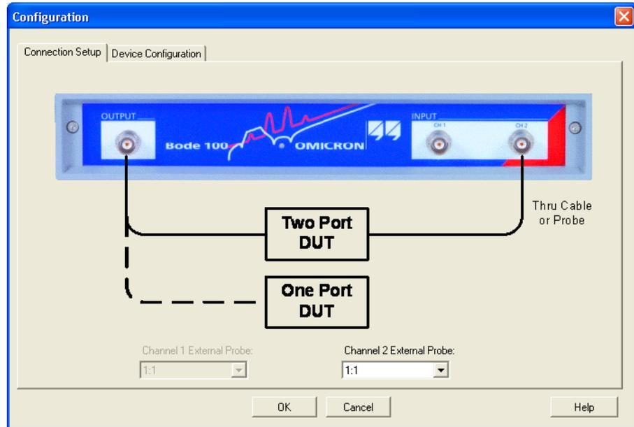
This picture shows you how to connect the DUT (quartz filter).
