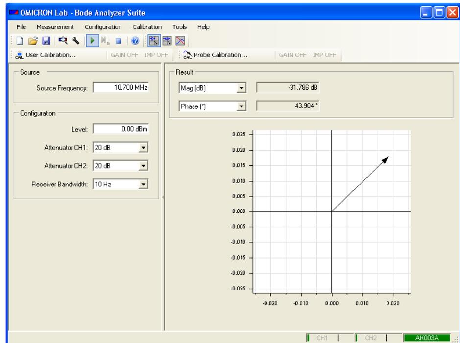
**Result:** The IF filter has a magnitude of  $-31.79$  dB at 10.7 MHz. Your result may differ because each IF filter is slightly different.
