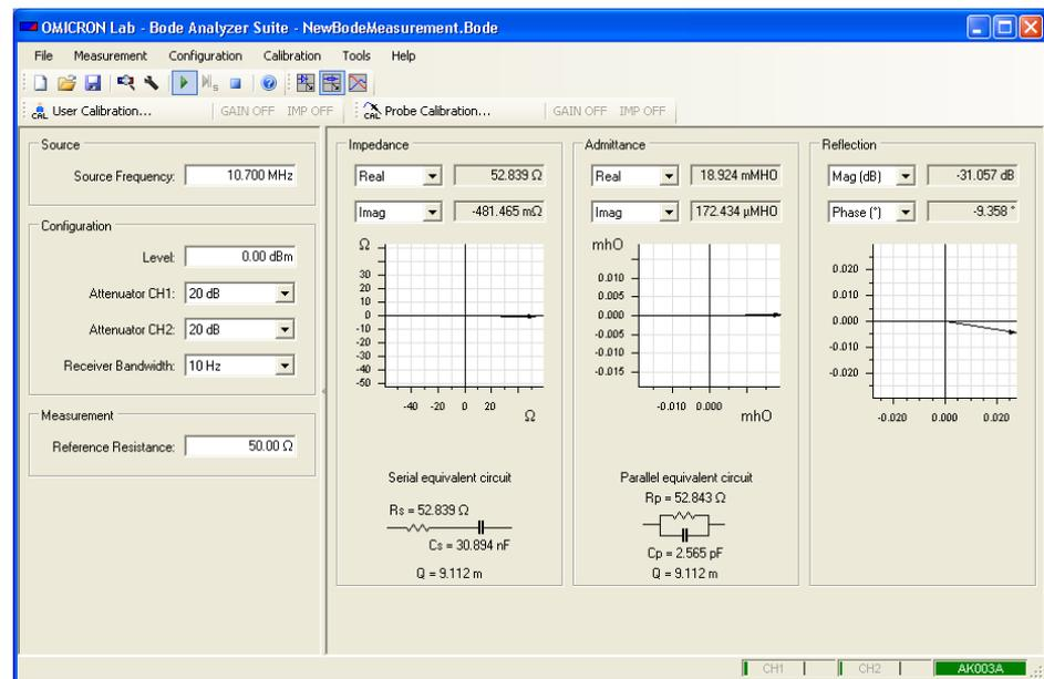
**Result:** The measured values of the IF filter at 10.7 MHz are:
