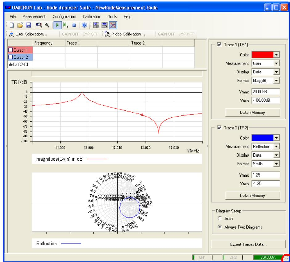
In the upper graph you see the gain of the quartz filter. You can use the cursors to measure the series and parallel resonance frequencies.
