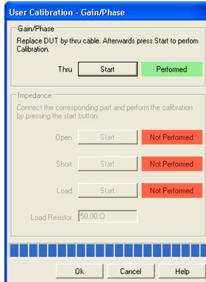
For the **Gain/Phase** measurement, the **Impedance/Reflection** calibration is not necessary. The **Gain/Phase** mode is now calibrated for the current specific measurement setup. Refer to 6.1 "Calibration Methods" on page 59 to learn in which cases you have to repeat the calibration if a parameter is changed.
