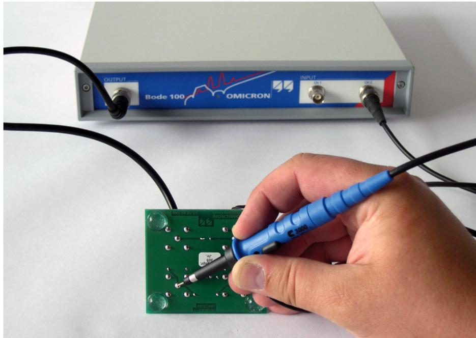
**Hint:** Ensure that the probe's tip is in contact with the DUT's input all the time until the calibration is finished.
