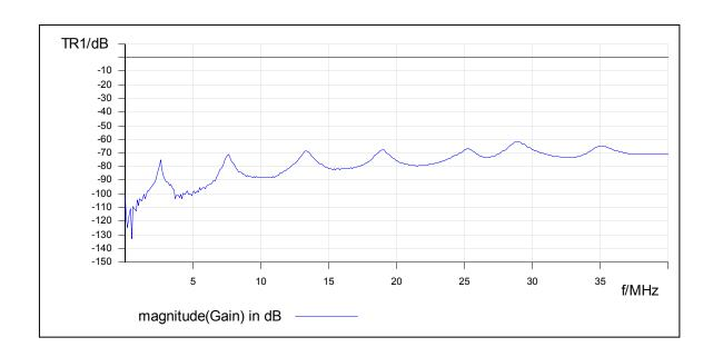
The curve shows the signal injected to our DUT (cable two). As you can see the screening is able to completely block the RF signal injected from cable one.
