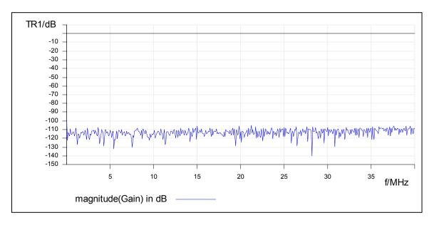
• As you can see in the chart above the isolation between the double shielded cables is much better (attenuation > 100dB)
