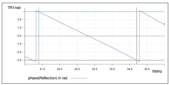
• Calculate the cable length ( $\Delta \Phi$  = -5.94 rad and  $\Delta f$  = 2.80 MHz)
