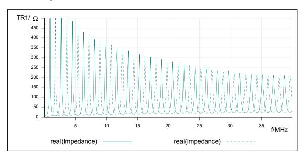
• Diagram for the measured impedance of a  $75\Omega$  cable (50 meters):
