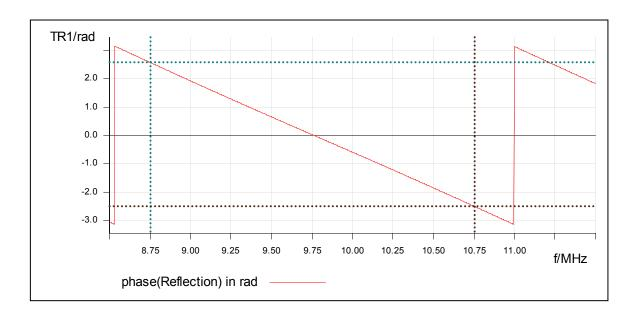
• The new values:  $\Delta \Phi = -5.07 \text{ rad}$  $\Delta f = 2.0 \text{ MHz}$
